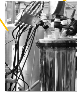
LHe cryostat with THz windows
